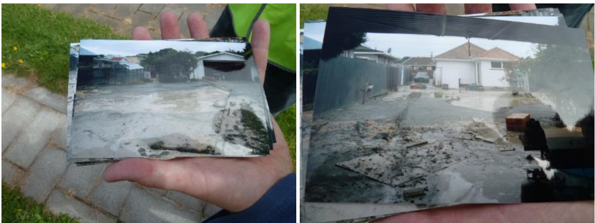
Figure 95: Ground photographs of the ejected material within Patch C.
